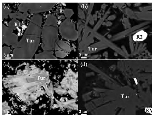
Fig. 1 - BSE images of REE-tourmalines (Tur), obtained at low pressure (2 kbar): (a) La-tourmaline and LaBSiO<sub>5</sub> (R1), (b) Nd-tourmaline and NdBSiO<sub>5</sub> (R2), (c) Eu-tourmaline, (d) Yb-tourmaline and Yb<sub>2</sub>(Si<sub>2</sub>O<sub>7</sub>) (KV).
