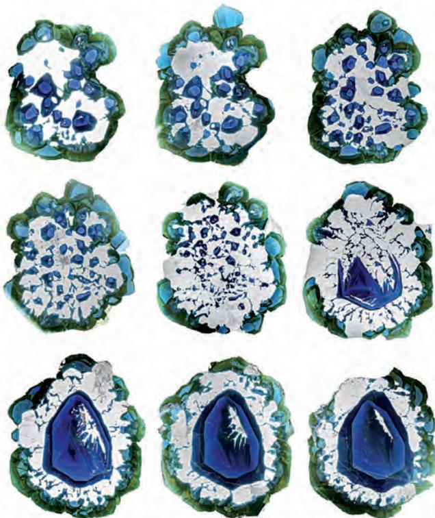
Fig. 11 - Crystallization shifted from skeleton growth forming the hollow center to dendritic growth (intergrowth with quartz). Finally the satellite crystals in the rim and on the top grew in normal mode. Crystal from Minas Gerais, diameter 2.5 cm.
