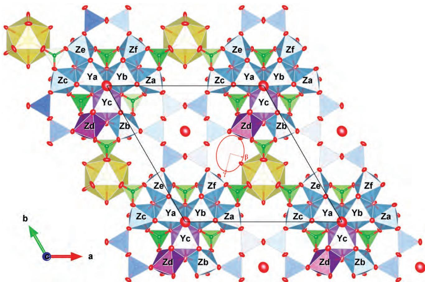
Fig. 2 - The [001] projection of the *R1* structure model showing the location of Yc and Zd sites (b). The direction of experimentally determined  $\gamma$  (and  $\beta$ ) directions is reported as the approximate acute bisectrix section of the optical indicatrix (in red).
