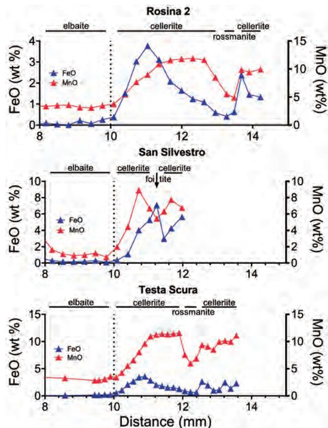
Fig. 3 - Variation in MnO and FeO (wt%) along a straight traverse parallel to the *c*-axis of three selected crystals, from the upper section to the dark termination. The dashed line marks the transition between the upper section and the dark colored termination of the crystals.
