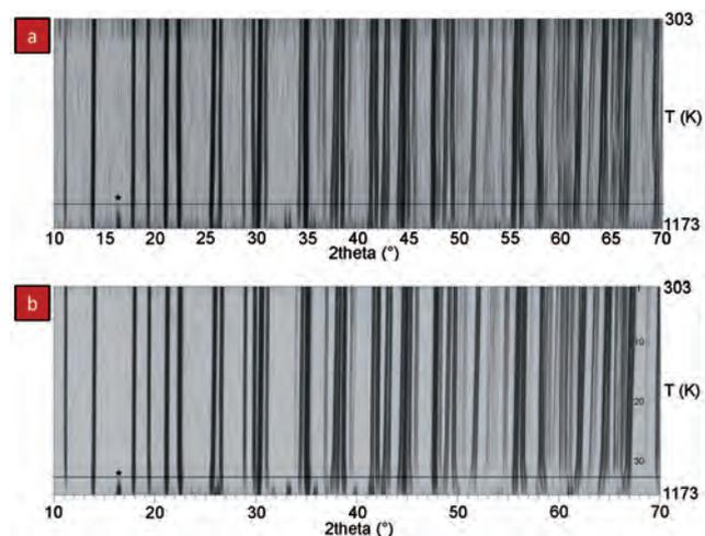
Fig. 1 - Pseudo-Guinier plot of XRPD data of Fe-rich fluor-elbaite a) and Mn-bearing elbaite b). The horizontal lines at 1076 and 1098 K (803 and 825 °C), respectively, represent the first occurrence of the B-mullite peaks, the most intense of which is marked by the “\*\*” symbol.
