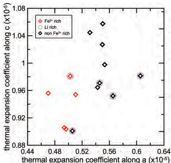
Fig. 1 - Thermal expansion along the *a* and *c* axes in the tourmalines studied. The Fe<sup>2+</sup>-poor tourmalines with the lower *c* expansion is the olenitic sample (namely, Vac-Al-B-rich elbaite).
