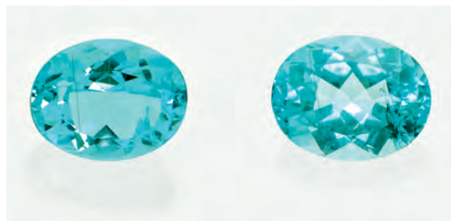
Fig. 3 - This 2.6 ct Paraíba-type tourmaline from Mozambique is shown as received for gem testing with oil-filled fissures (left), and after the oil has been removed from the fractures by cleaning the stone in acetone (right). (Composite photo © SSEF).
