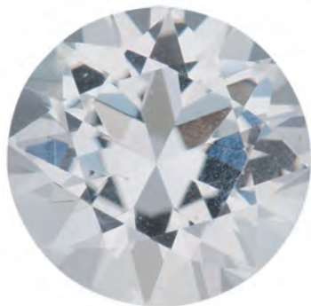
Fig. 2 - 3.34 ct colorless "liddicoatite" with extremely high Pb (17400 ppmw) and Mn (23400 ppmw) concentration, courtesy of Bruce A. Fry. Photo © GIA.
